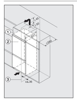
The appliance can be installed in a kitchen run. To match the height of the rest of the kitchen, the appliance can be fitted with a suitable top box ①.
